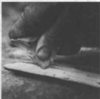
...then gouging a depression to start the hole.
