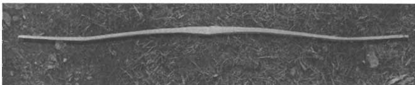
#4—Showing how bow somewhat followed string from just one time stringing
